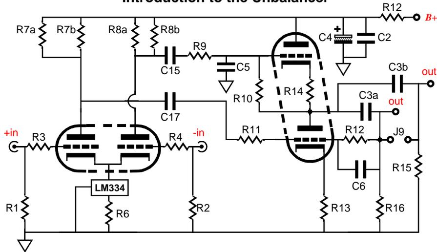
**Unbalancer Topology** The Unbalancer circuit accepts a balanced input signal and delivers an unbalanced, single-ended output. Besides performing the conversion, the Unbalancer circuit provides voltage gain and exhibits a fine CMRR (Common Mode Rejection Ratio), which means that it largely ignores common-mode signals. Balanced signals offer some real advantages, such as lower noise and easy phase reversal and no need for a phase splitter, in a push-pull power amplifier.
